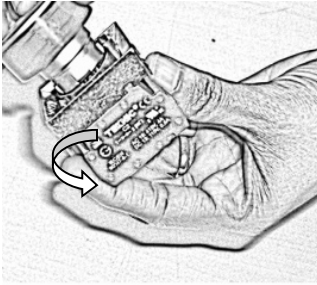
Turn the actuator in anticlockwise direction
