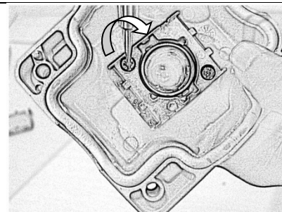
Tighten the lock screw with a torque of 1.2Nm
